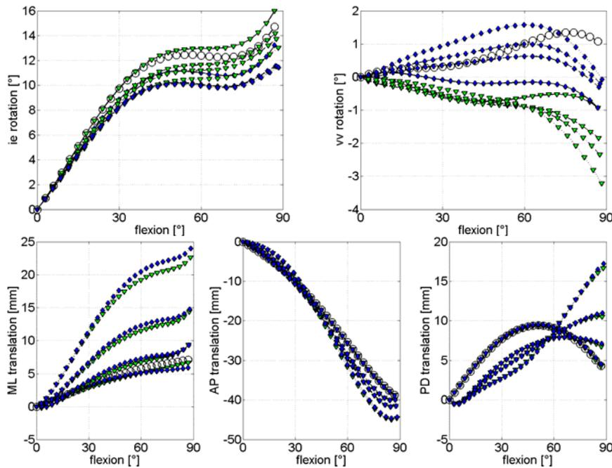
**Figure 3: 6 DOF joint displacement for a maximum marker perturbation due to STA: 0 mm (solid lines), shank: 1 mm / thigh: 3 mm (dashed lines), 5 mm/15 mm (dash-dotted lines), 10 mm/30 mm (dotted lines).**
