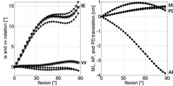
**Figure 2: 6 DOF displacement in the absence of data perturbations.**  $\circ$ : Input 6 DOF displacement.  $\blacksquare$ : data related to the original flexion axis;  $\blacktriangledown$ : data related to SARA axis,  $\blacklozenge$ : data related to FHA.
