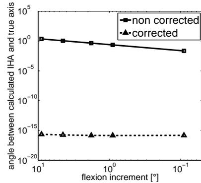
Fig. 1. IHA calculation: Due to discretization errors depending on the angular step width the calculated axis direction deviates from the true axis direction. Squares (■) depict this effect for pure flexion data when the IHA formulas are not corrected, triangles (▲) depict the corrected version.
