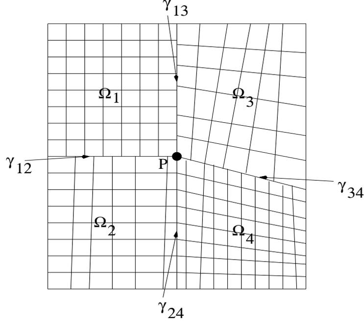
FIGURE 1. The domain  $\Omega$  is partitioned into four subdomains  $\Omega_i$   $i = 1, 2, 3, 4$  with interfaces  $\gamma_{ij}$ ; each subdomain is partitioned into quadrilateral finite elements independently;  $P$  is a cross point
