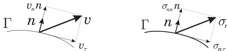
FIGURE 1. Normal and tangential components of a vector v and normal tensor component \sigma_n with respect to the manifold \Gamma .
