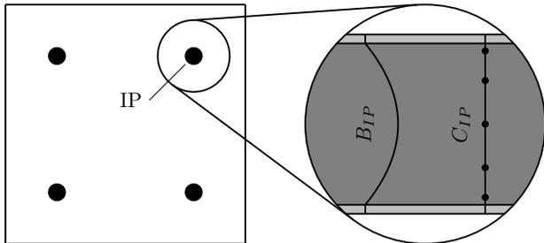
Fig. 2. In each integration point IP the corresponding  $\mathbf{B}$  field in  $z$  direction is reconstructed and numerical integration is carried out for the terms containing the nonlinear parameter  $\mu$ .
