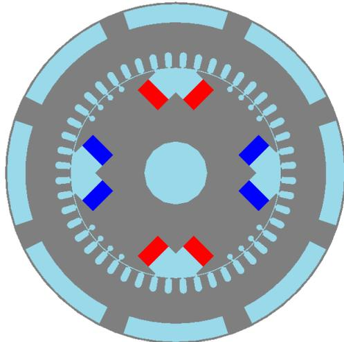
Fig. 1. The cross section of the machine  $\Omega_{2D}$ . The materials are iron (grey) and air (light blue). The coils are visualized in red and blue, indicating a positive (red) or negative (blue) d.c. current density.
