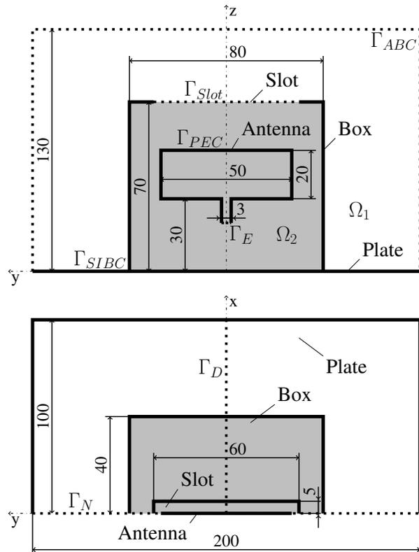
Fig. 1. Geometry of a small loop antenna located in a metallic box with a slot. Cutaway front view (top) and top view (bottom). The cut has been made in the symmetry plane  $\Gamma_N(x = 0)$ . The second symmetry plane is  $\Gamma_D(y = 0)$ . All measurements are given in millimeters (mm). The antenna has a diameter of 1mm.
