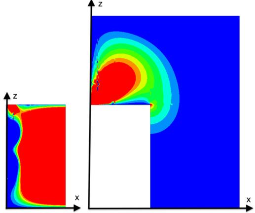
Fig. 3. B-field inside (left) and outside (right) of the box in a plane parallel to the x-z-plane. The real part of the z-component of the B-field is visualized. The box and the metallic plate are modeled as PEC. The external field is multiplied by a factor of 10.
