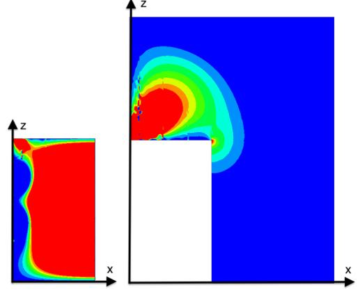
Fig. 2. B-field inside (left) and outside (right) of the box in a plane parallel to the x-z-plane. The real part of the z-component of the B-field is visualized. SIBC is applied on the box and metallic plate. The external field is multiplied by a factor of 10.
