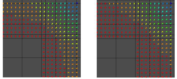
Fig. 4. Imaginary part of the current density at  $y = \text{const.}$  and  $f = 50$ Hz, RS (left), MSFEM (right).
