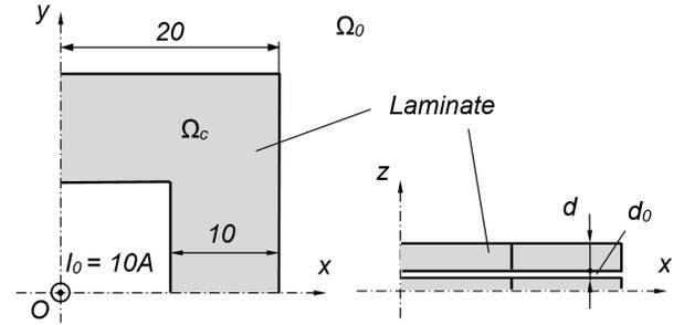
Fig. 1. Eddy current problem, problem not drawn to scale, top view (left) and front view (right), dimensions are in mm, origin  $O$  at  $(0,0,0)$ , planes of symmetry are  $x = 0$ ,  $y = 0$  and  $z = 0$ , quadratic structure in the  $xy$ -plane.
