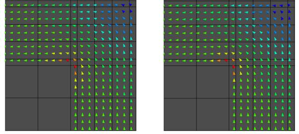
Fig. 3. Real part of the magnetic flux density at  $y = \text{const.}$  and  $f = 50$ Hz, RS (left), MSFEM (right).
