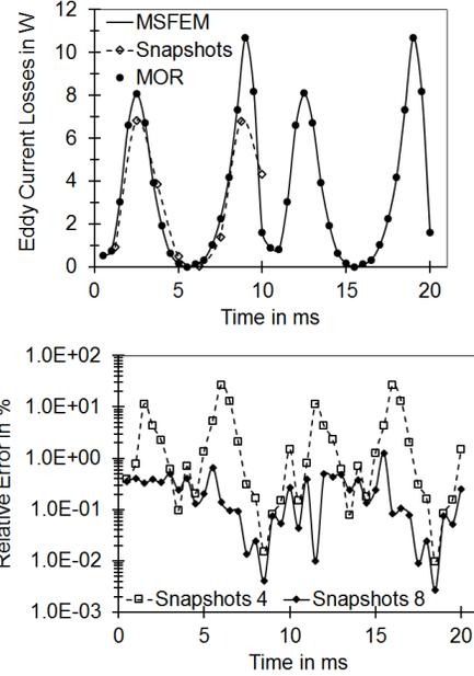
Fig. 2. Eddy current losses with  $I = 1A$  (above) and with 8 snapshots. Relative errors (below) for 4 and 8 snapshots.
