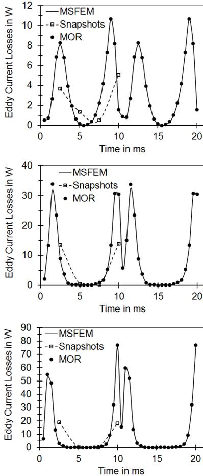
Fig. 1. Eddy current losses for different input currents  $I=1A$  (top),  $I=2A$  (middle) and  $I=3A$  (bottom) at frequency of  $f=50Hz$ .
