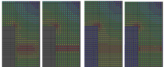
Fig. 2. Field distributions in a neighboring iron sheet next to the air gap: Eddy currents (first two), magnetic flux density (second two), reference solution (left) and MSFEM (right) in each case, only one quarter is shown, the same scaling of the respective results holds.
