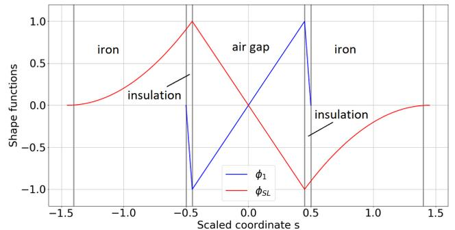
Fig. 1. Shape functions, the width corresponds to 3 iron sheets with 2 insulation layers in between. The period of  $\phi_1$  is 1.0, that of  $\phi_{SL}$  is 3.0 in scaled coordinates.
