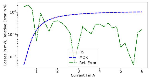
Fig. 2. Losses and relative error obtained by RS and by MOR.
