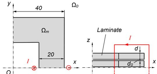
Fig. 1. Numerical example, problem not drawn to scale, origin  $O$  at  $(0,0,0)$ ,  $x = 0$ ,  $y = 0$  and  $z = 0$  represent planes of symmetry, top view (left) and front view (right) of one eighth with four laminates, dimensions are in mm, the structure is quadratic in the  $xy$ -plane, rectangular  $(30 \times 15)$  current loops are linked symmetrically with the limbs,  $d + d_0 = 0.25 \text{mm}$  selected with 2.5% fill factor.
