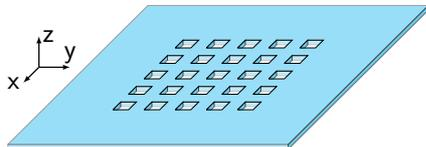
Fig. 1. Metascreen with small periodic apertures.
