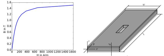
Fig. 1. The dimensions of the sheet are given as  $l = 30$  mm,  $w = 6$  mm,  $d = 0.5$  mm (5% of which are the air gap). The dimensions of the hole are  $1.2 \times 3$  mm. The electric conductivity  $\sigma$  is equal to  $2.08 \cdot 10^6$  S/m.
