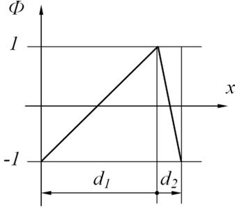
Fig. 2. Periodic micro-shape function  $\phi(x)$
