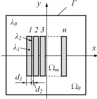
Fig. 1. Draft of the boundary value problem with a laminated medium, top view
