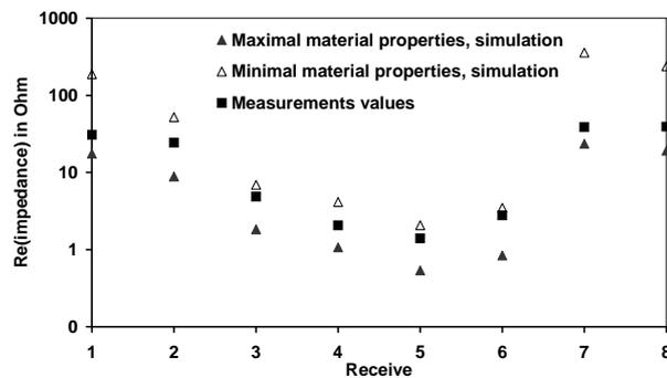
Fig. 3: Real part of the impedances of test person A for varying material properties.
