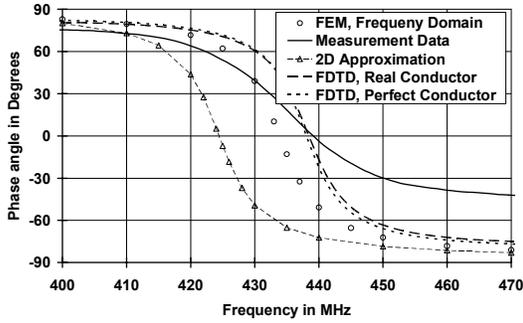
Figure 3: Phase angle as a function of the excitation frequency.
