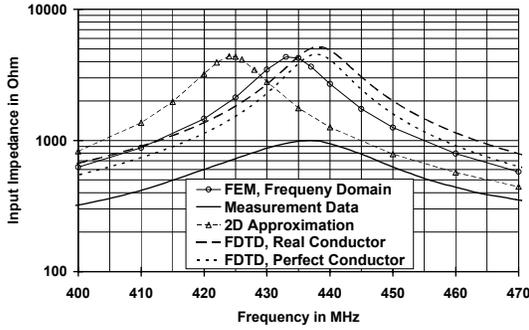
Figure 2: Input impedance as a function of the excitation frequency.
