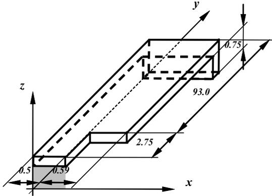
Figure 1: One fourth of the microstrip, all dimensions are in millimeter, thickness of the conductor equals to  $35.0 \cdot 10^{-3} \text{ mm}$ .
