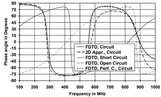
Figure 5: Phase angle as a function of the excitation frequency.
