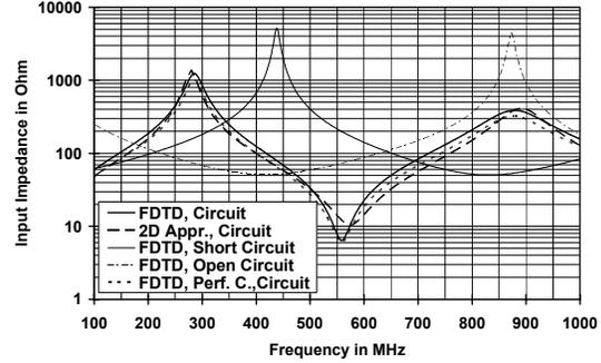
Figure 4: Input impedance as a function of the excitation frequency.
