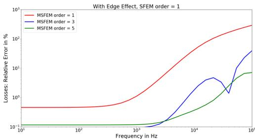
Fig. 12. The relative error of the eddy current losses versus frequency of higher order 2D/1D MSFEMs with EE.
