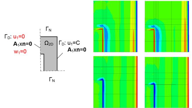
Fig. 9. Boundary conditions for  $u_1$ ,  $\mathbf{A}_1$  and  $w_1$ ,  $\Gamma_D \cup \Gamma_N = \partial\Omega_{2D}$ , hole is included in  $\Omega_{2D}$  (left). Current densities in the vicinity of the hole in the plane of symmetry at  $z = 0.0$ , 2/1D MSFEM with EE, entire problem (middle) and one quarter (right):  $z$ -components  $Re\{J_z\}$  (above) and  $Im\{J_z\}$  (below),  $f = 1,000Hz$ .
