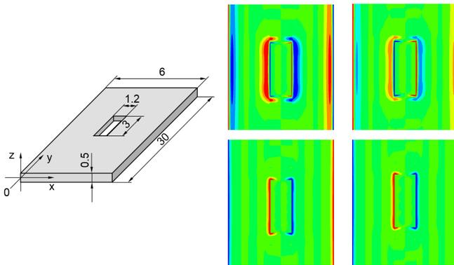
Fig. 7. Laminate with a hole, dimensions in mm (left). Current densities in the vicinity of the hole in the plane of symmetry at  $z = 0.0$ , 3D SFEM (middle) and the 2D/1D MSFEM with EE (right):  $z$ -components  $Re\{J_z\}$  (above) and  $Im\{J_z\}$  (below),  $f = 1,000Hz$ .
