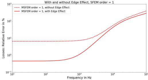
Fig. 10. The relative error of the eddy current losses versus frequency of the linear 2D/1D MSFEMs.
