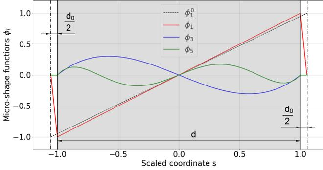
Fig. 3. Micro-shape functions, the grey interval  $[-1, 1]$  represents the iron laminate and beyond that up to the dash-dotted line there is the air gap.
