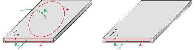
Fig. 2. Magnetic fields and eddy currents in general associated with a laminate (left), without stray field  $B_s$  and currents  $J_s$  and without edge effect (right).
