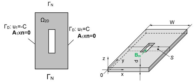
Fig. 6. Boundary conditions for  $u_1$  and  $\mathbf{A}_1$  representing a flux tube.
