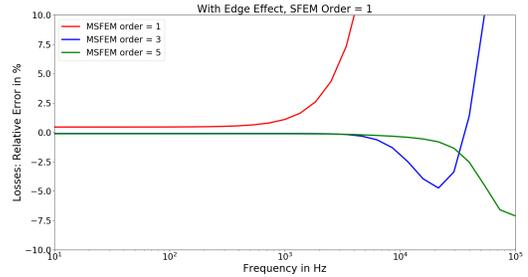
Fig. 13. The relative error of the eddy current losses versus frequency of higher order 2D/1D MSFEMs with EE, linear scale of the error, detail.
