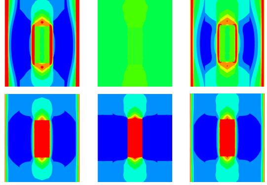
Fig. 8. Current densities in the vicinity of the hole in the plane at  $z = 1.8mm$ , 3D SFEM (left), the 2D/1D MSFEM without EE (middle) and the 2D/1D MSFEM with EE (right):  $x$ -components  $Re\{J_x\}$  (above) and  $Im\{J_x\}$  (below),  $f = 1,000Hz$ .
