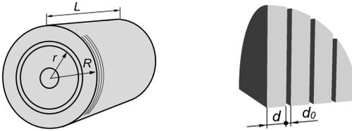
Fig. 1. Large scale: electrical machine with overall dimensions  $L$ ,  $R$  and  $r$ , lamination is indicated (left). Fine scale: thickness  $d$  of the laminates and the width  $d_0$  of the air gaps (right).
