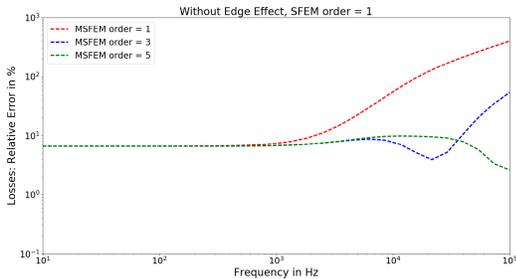
Fig. 11. The relative error of the eddy current losses versus frequency of higher order 2D/1D MSFEMs without EE.
