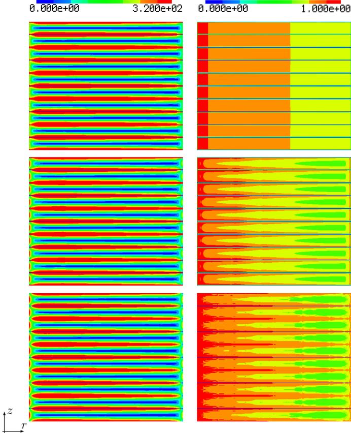
Fig. 12. Absolute value of the  $J$  (left) and  $B$  (right) field at  $t = 17.2\text{ms}$  for (from top to bottom) the first order MSFEM, third order MSFEM and the reference solution, using the Preisach model at 50 Hz and an average flux density of 1.2 T.
