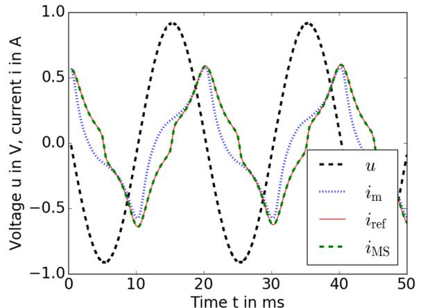
Fig. 7. Comparison of the current  $I$  at a given voltage  $U$  for the measurement data (m), the FEM reference solution (ref) and the multiscale solution (MS) for an average flux density of 1.2 T, using the nonlinear B-H curve at 50 Hz.
