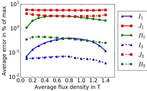
Fig. 13. Average errors of the MSFEM solution compared to the reference solution over a range of average flux densities using the nonlinear B-H curve at 50 Hz, for both the 1<sup>st</sup> order and 3<sup>rd</sup> order MSFEM.
