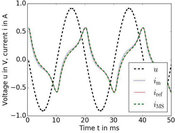
Fig. 8. Comparison of the current  $I$  at a given voltage  $U$  for the measurement data (m), the FEM reference solution (ref) and the multiscale solution (MS) for an average flux density of 1.2 T, using the Preisach model at 50 Hz.
