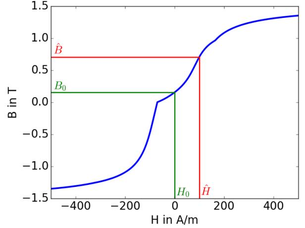
Fig. 4. The B-H curve obtained by the initial point  $(H_0, B_0)$  and a certain history, varying the input  $H$ . The history was artificially chosen to accentuate the discontinuities in the first derivative.
