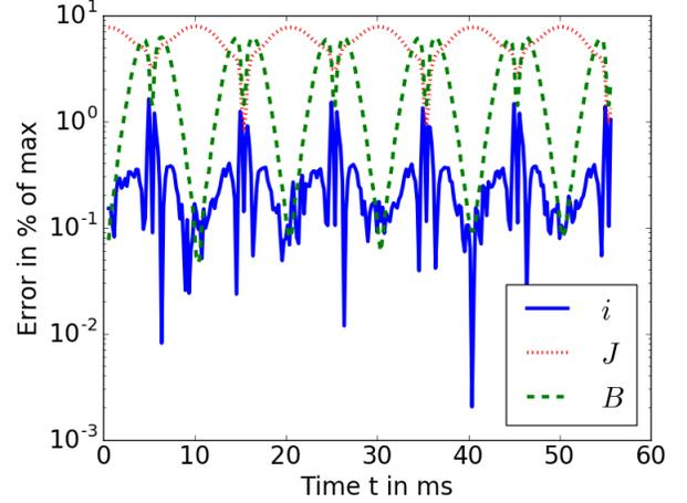
Fig. 10. The errors of the first order MSFEM solution to the reference solution at an average flux density of 1.2 T, using the nonlinear B-H curve at 50 Hz.
