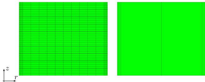
Fig. 5. The mesh for the reference solution (918 elements) and the multiscale solution (6 elements).
