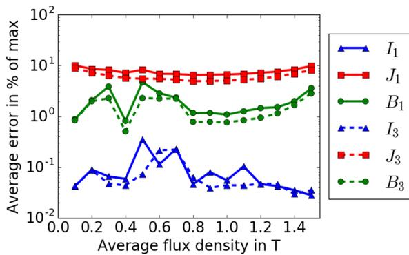
Fig. 16. Average errors of the MSFEM solution compared to the reference solution over a range of average flux densities using the Preisach model at 10 Hz, for both the 1<sup>st</sup> order and 3<sup>rd</sup> order MSFEM.
