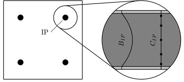
Fig. 3. Each integration point IP in each finite element is assigned a one dimensional reference cell  $C_{IP}$  consisting of the iron sheet (dark gray) and the air gap (light gray). The field  $B_{IP}$  and the coefficients derived from it are averaged using numeric integration.
