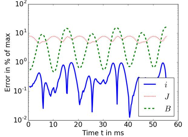
Fig. 11. The errors of the first order MSFEM solution to the reference solution at an average flux density of 1.2 T, using the Preisach model at 50 Hz.
