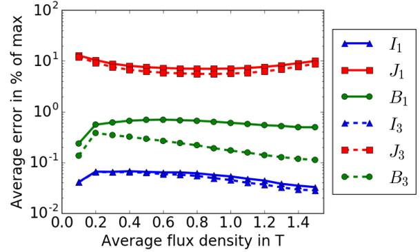
Fig. 15. Average errors of the MSFEM solution compared to the reference solution over a range of average flux densities using the nonlinear B-H curve at 10 Hz, for both the 1<sup>st</sup> order and 3<sup>rd</sup> order MSFEM.
