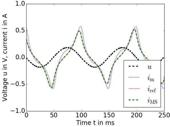
Fig. 9. Comparison of the current  $I$  at a given voltage  $U$  for the measurement data (m), the FEM reference solution (ref) and the multiscale solution (MS) for an average flux density of 1.2 T, using the Preisach model at 10 Hz.
