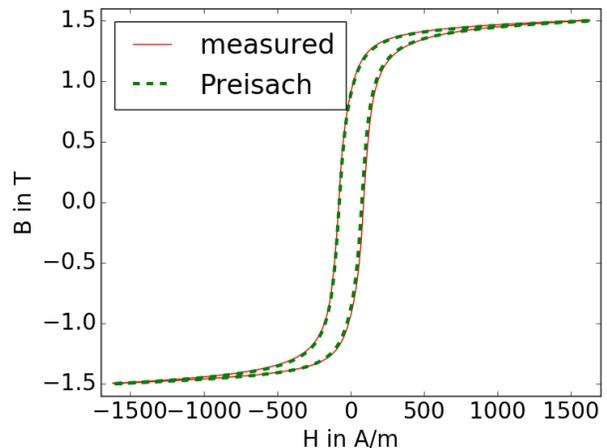
Fig. 6. Comparison of the measured major hysteresis loop and the approximation at 50 Hz.
