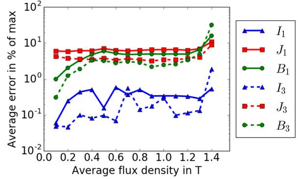
Fig. 14. Average errors of the MSFEM solution compared to the reference solution over a range of average flux densities using the Preisach model at 50 Hz, for both the 1<sup>st</sup> order and 3<sup>rd</sup> order MSFEM.
