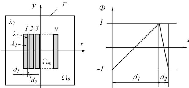
Fig. 1. Boundary value problem with a laminated media, top view (left) and periodic micro-shape function  $\phi(x)$  (right).
