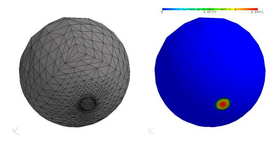
As mentioned above, the mixed form and the derived algorithm are also well suited for body-body contact problems. Preliminary results are available by B. Hackl and W. Hinterberger, more details can be found in [12]. Two rolls are in contact along a small strip. The smaller roll is loaded by given surface traction, and it is asked for its vertical displacement. The adaptive mesh with 46611 Nodes and the isosurface of the von-Mises stress is drawn below:
