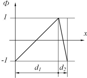
Fig. 5. Periodic micro-shape function  $\phi(x)$ , one periode is shown.
