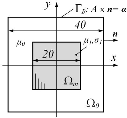
Fig. 11. Numerical example of an eddy current problem, dimensions in mm.
