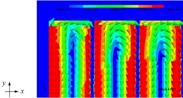
Fig. 12. Detail of the eddy current distribution in laminations in the upper left corner, homogenized solution.
