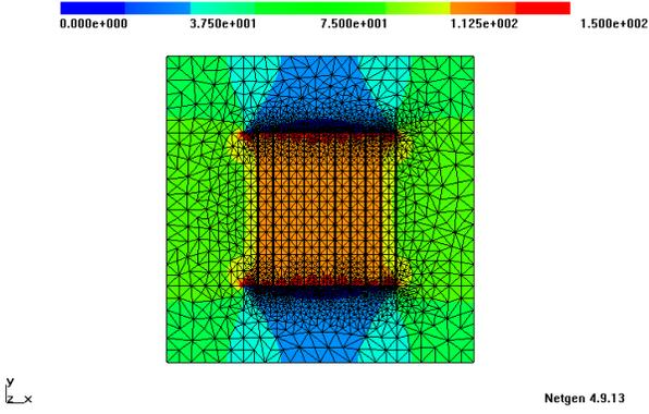
Fig. 7. Flux density of the reference problem: x-component.
