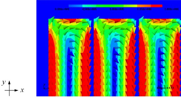
Fig. 10. Detail of the eddy current distribution in laminations in the upper left corner, reference solution.
