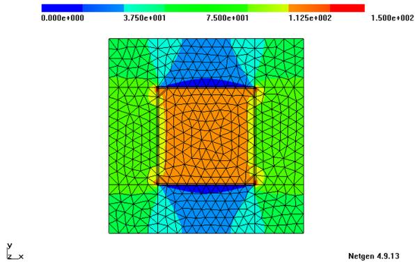
Fig. 8. Flux density of the homogenized problem: x-component.
